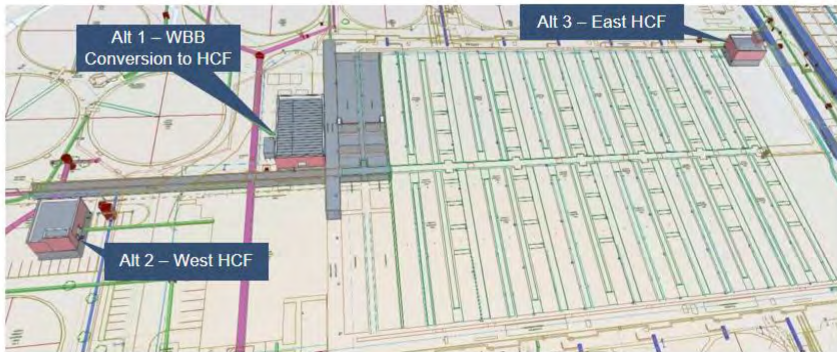
Figure 2 - Potential Site Locations for Hydrocyclone Facility
