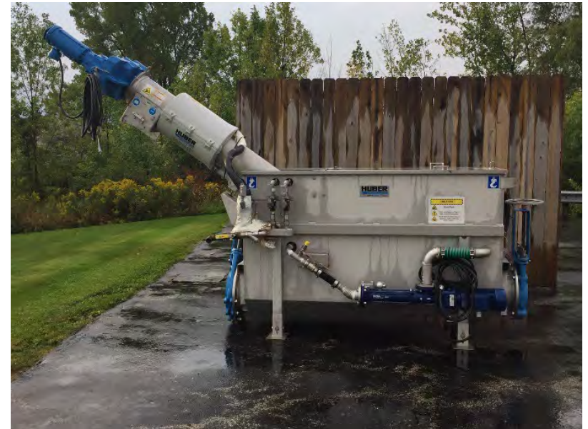
Huber Drum Screen Pilot Unit
