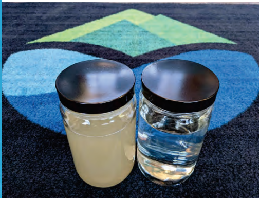
NTP untreated influent (left) compared to treated effluent (right) in May.
